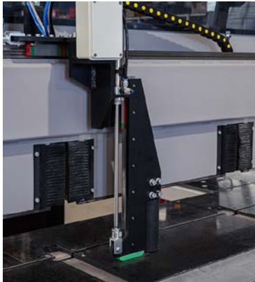
Automatic Side Aligner The side aligner runs on prismatic guides and ensures precision on cross-way cuts. Powerful pusher for panel movement. The pusher travels through precision pinions and racks. Maximum accuracy thanks to double measuring system: magnetic encoder and servomotor.
