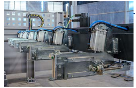
Pneumatic mechanism for the safe separation of panels from the stack.
