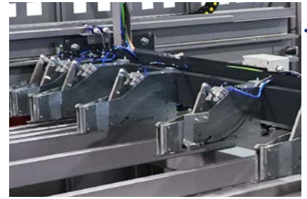
Double-piston grippers with removable down finger which ensure perfect transport of the selected panels from the stack without damage.
