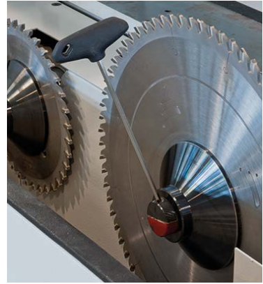
Practical and reliable blade change system (easy change) by using only 1 key
