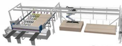
Automated magazine – panel storage system
