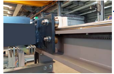
Heavy duty (H) beams pusher movement by rack - pinion system (Atlanta). Smooth movement without vibrations.
