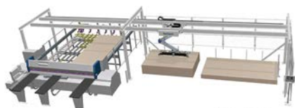
Automated magazine – panel storage system
